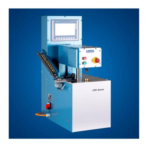
The automatic cylinder calibration machine ZPM is used for machining tungsten carbide drawing dies in the smaller boring diameter range 0.13 to 2.00 mm. By rotation and oscillation, the cylinder is incorporated and simultaneously polished. Using special calibration wires, dies can be manufactured with an accuracy of up to +/- 0.001 mm.
